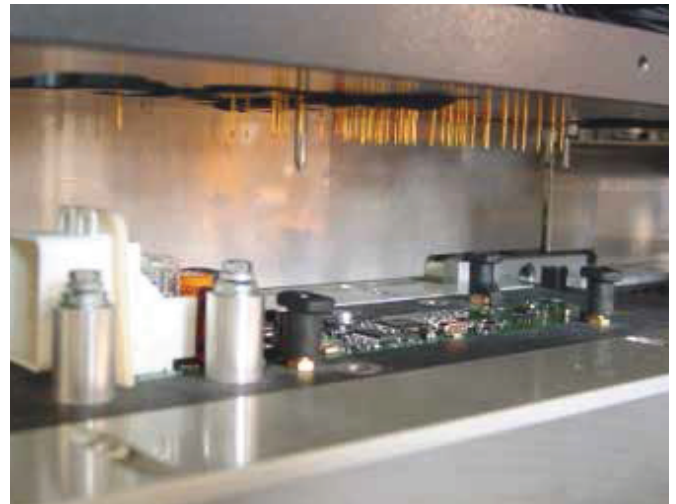
Contacting system for HFT
