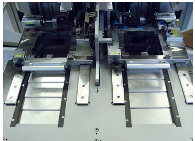
Leakage test machine offline (two test rigs)
